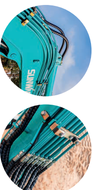
Extra protection for hoses / AUX 2 lines
